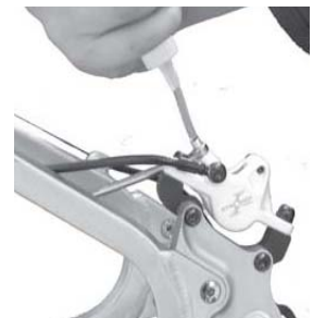
(Fig. 5) Attach the fluid bottle to the caliper bleeder
