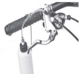
(Fig. 4) Remove the bleed screw and attach the catch container.
