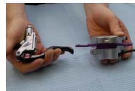
(Fig. 6) Align caliper pistons using Slot Slug tool.
