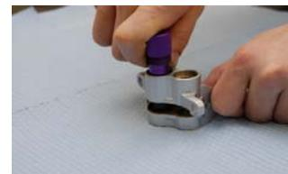
(Fig. 2) Remove the outboard caliper pistons.
