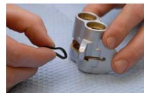
(Fig. 5) Install the caliper square seals.
